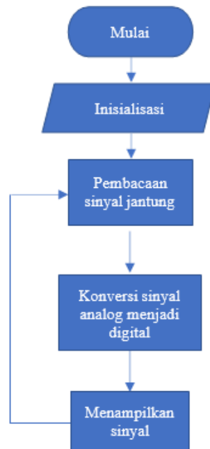
Gambar 3 Flowchart Sistem Elektrokardiogram
