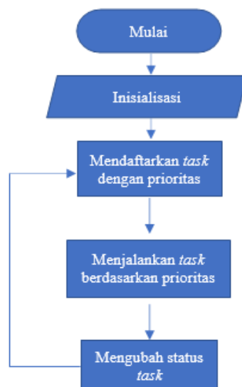
Gambar 4 Flowchart Real-time Operating System
