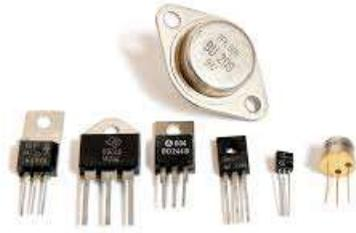
Gambar 1 Transistor
