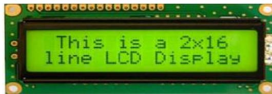
Gambar 2. LCD 16 x 2 (Hafidhin et al., 2020)
