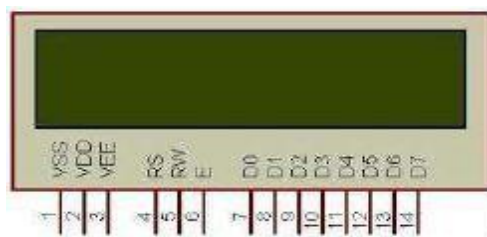
Gambar 3. LCD Monitor 16 x 2 (S Samsugi, 2017)
