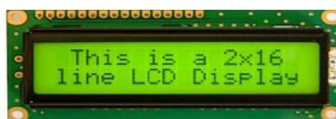
Gambar 3 LCD 16 x 2 (Sintaro et al., 2021)
